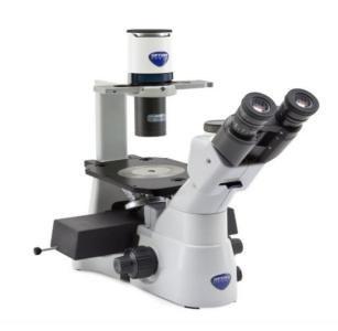
Inverted trinocular LED fluorescence microscope, B & G LED Fluorescence Cubes, IOS LWD W-PLAN PH objectives
